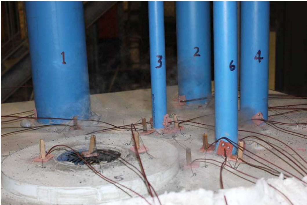
PHOTOGRAPH 4 – SPECIMENS AFTER 120 MINUTES OF TESTING
