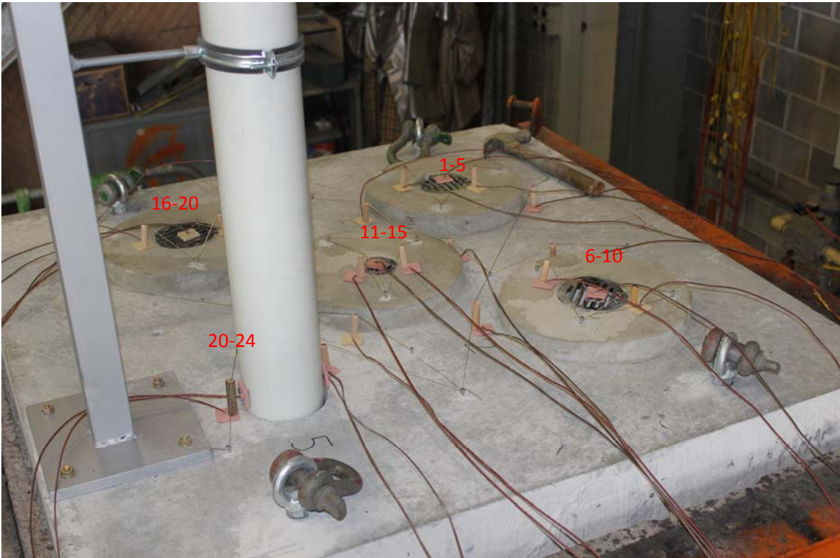
PHOTOGRAPH 2 – UNEXPOSED FACE OF SPECIMENS PRIOR TO TESTING
