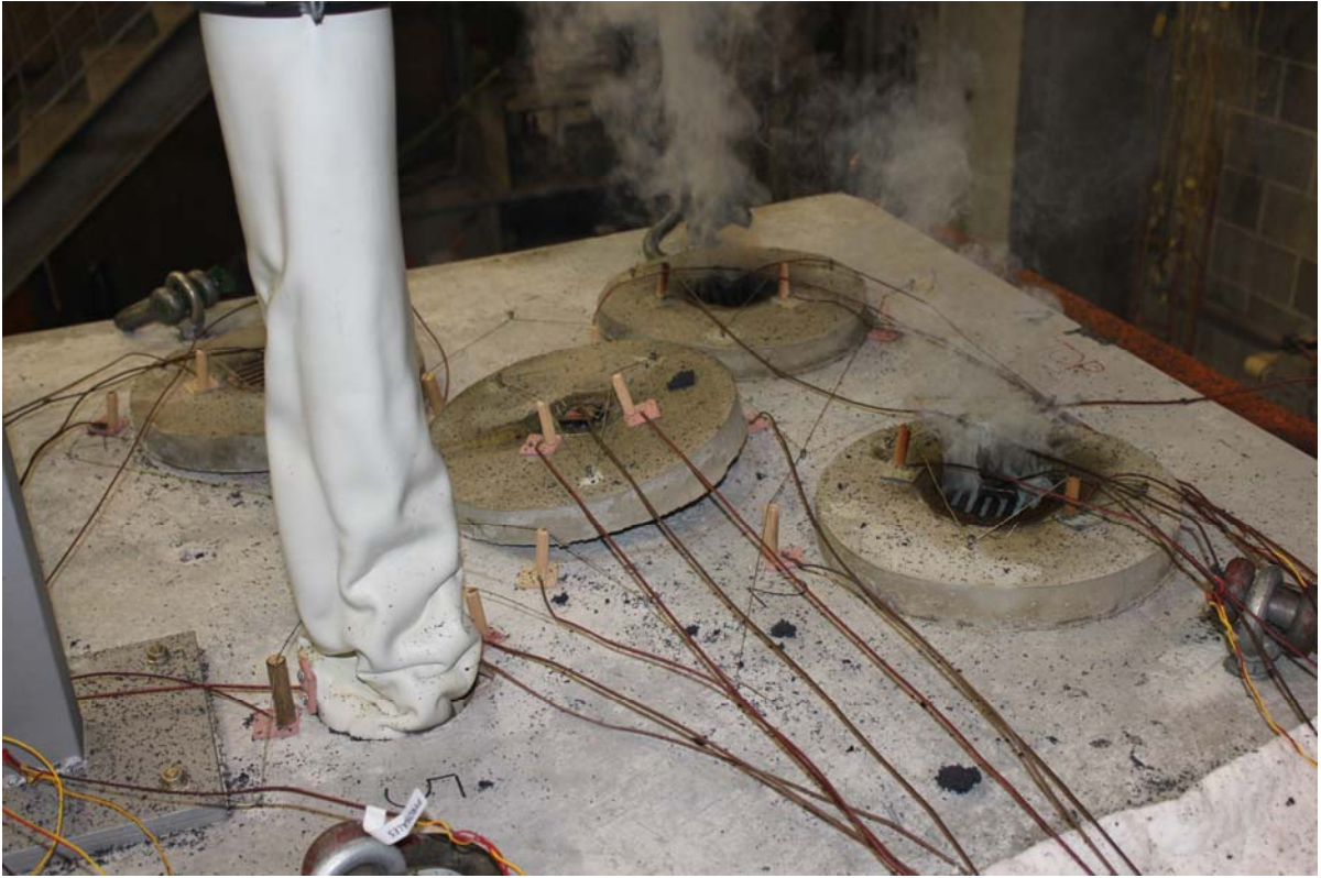
PHOTOGRAPH 5 – SPECIMENS AFTER 180 MINUTES OF TESTING
