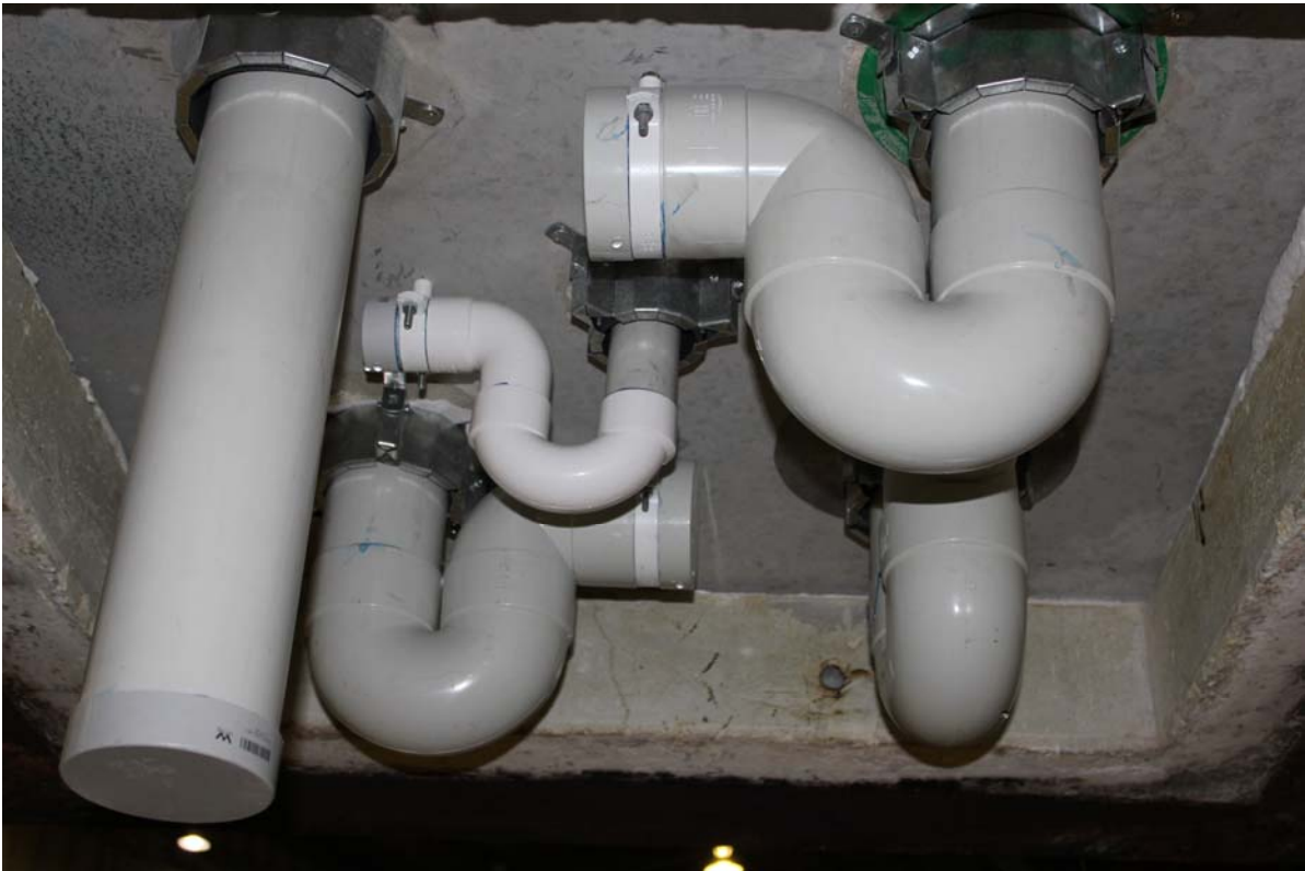
PHOTOGRAPH 1 – EXPOSED FACE OF SPECIMENS PRIOR TO TESTING
