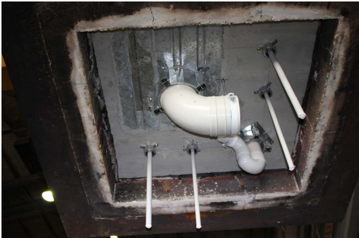
PHOTOGRAPH 2 – EXPOSED FACE OF SPECIMEN PRIOR TO TESTING
