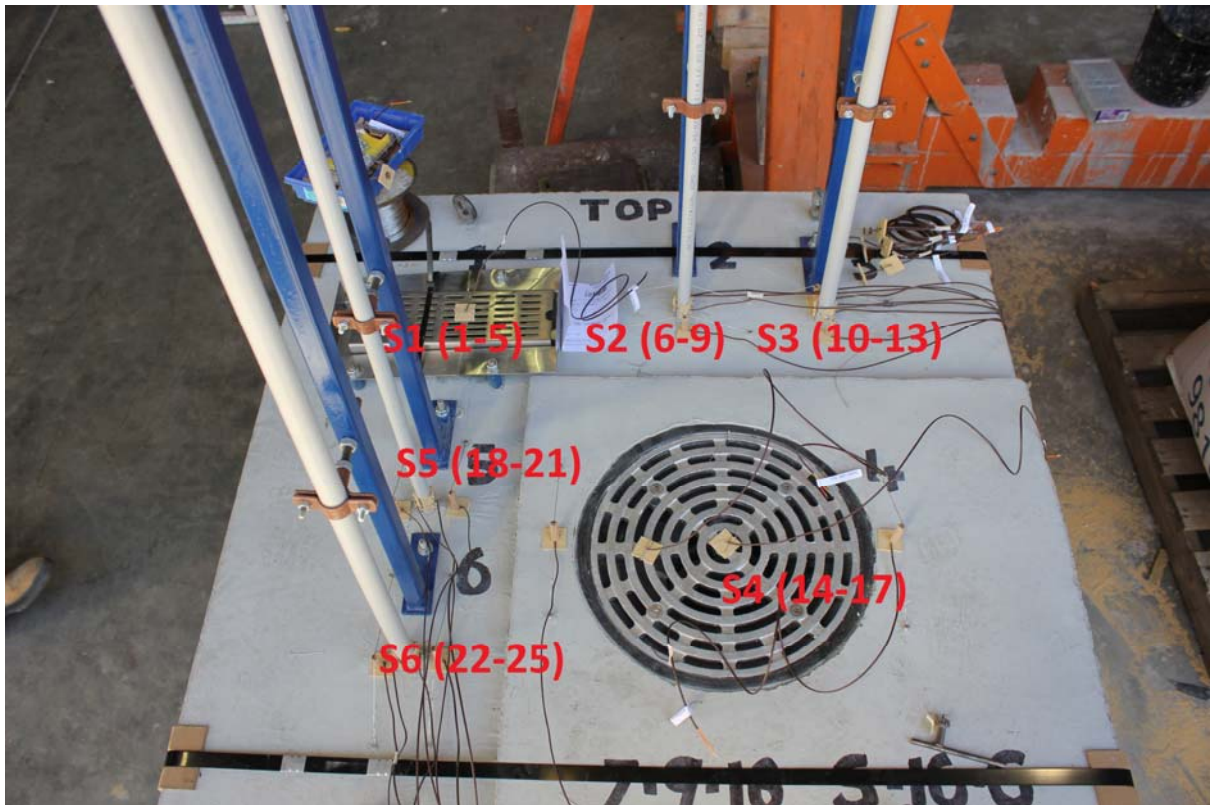
PHOTOGRAPH 1 – UNEXPOSED FACE OF SPECIMENS PRIOR TO TESTING
