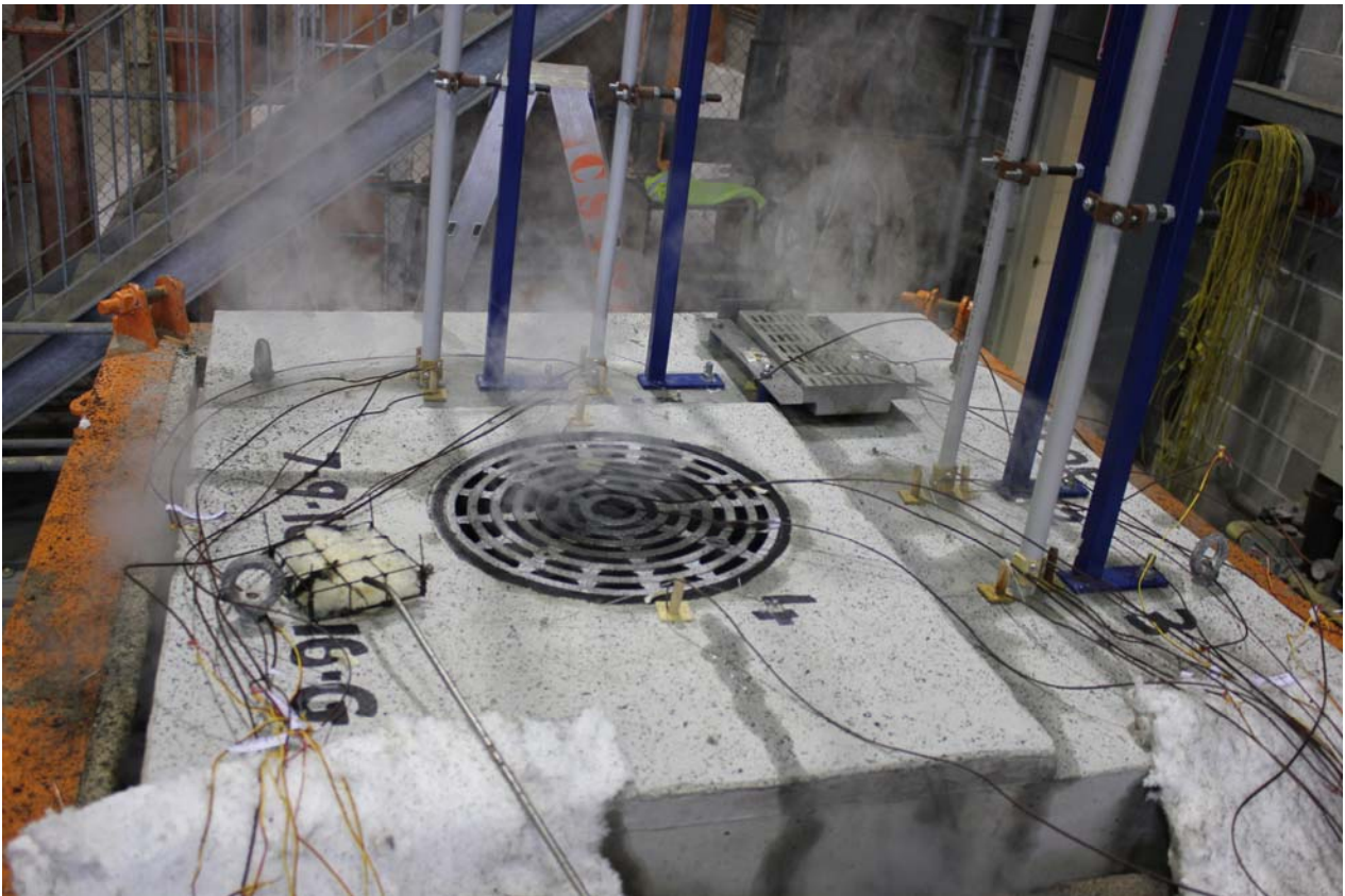
PHOTOGRAPH 3 – SPECIMENS AFTER 60 MINUTES OF TESTING
