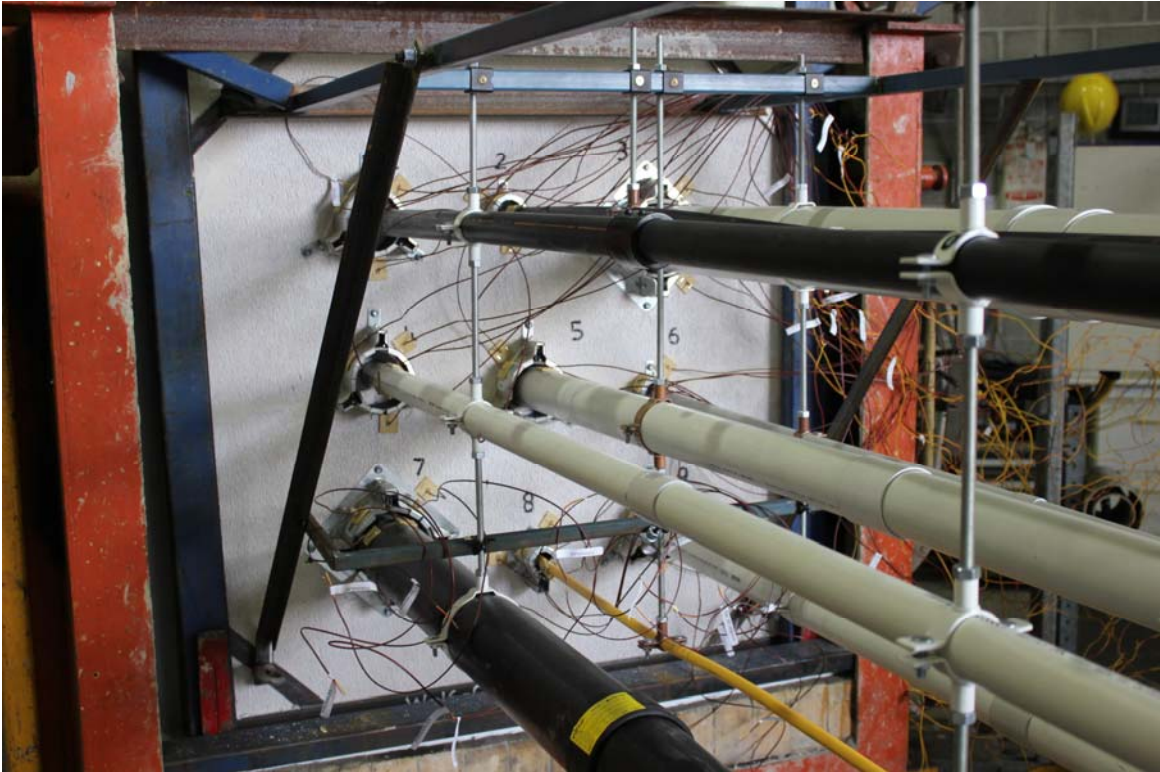
PHOTOGRAPH 1 – UNEXPOSED FACE OF SPECIMENS PRIOR TO TESTING
