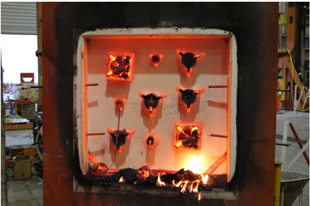
PHOTOGRAPH 4 – EXPOSED FACE OF SPECIMENS AT CONCLUSION OF TESTING
