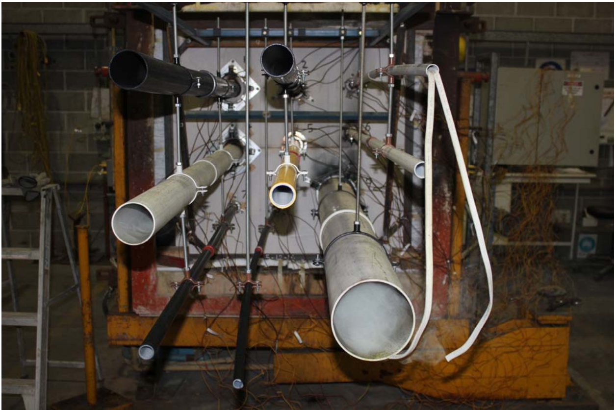
PHOTOGRAPH 3 – SPECIMENS AFTER 120 MINUTES OF TESTING
