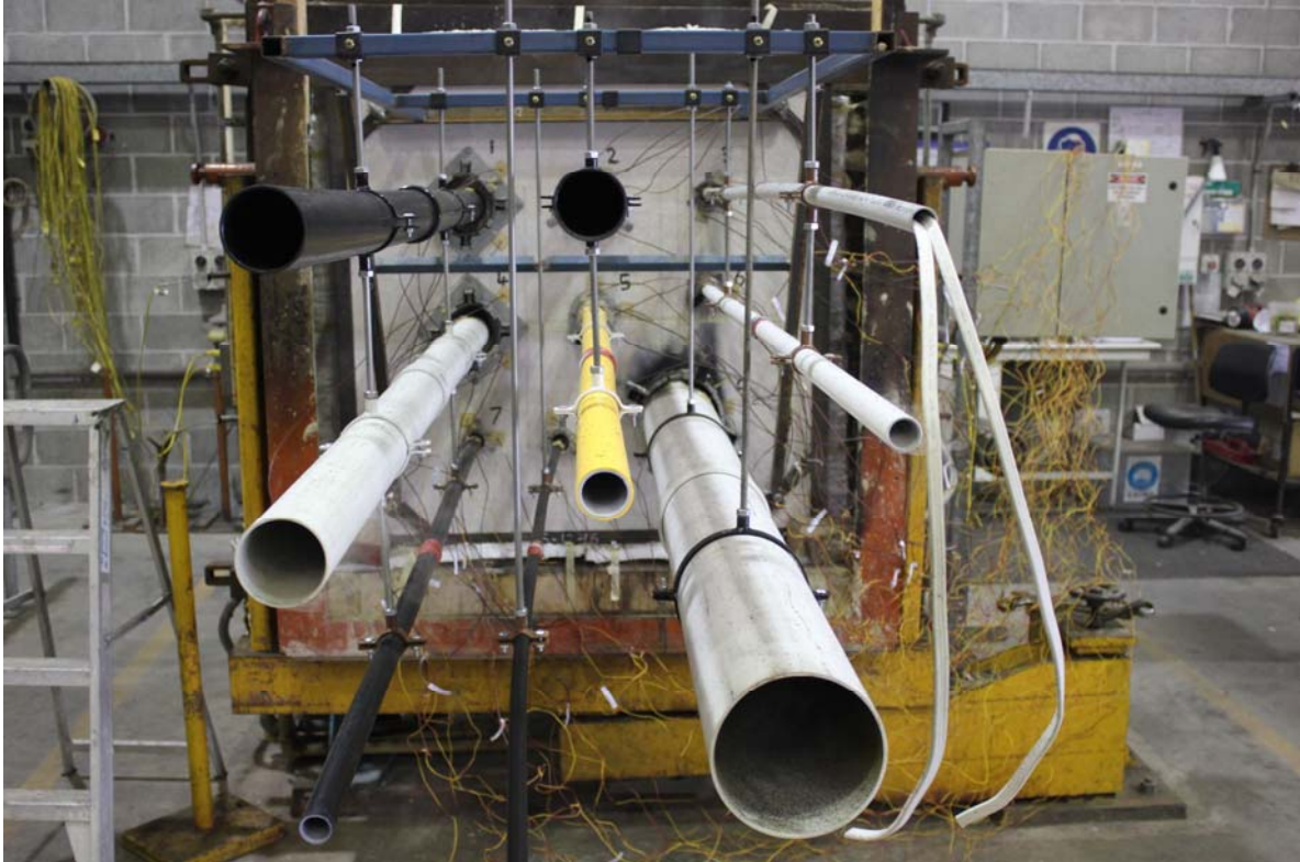
PHOTOGRAPH 2 – SPECIMENS AFTER 60 MINUTES OF TESTING
