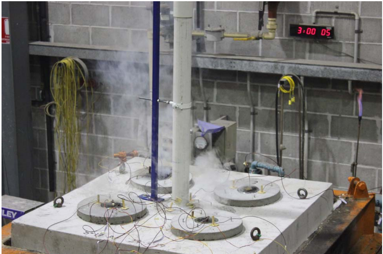
PHOTOGRAPH 5 – SPECIMENS AFTER 180 MINUTES OF TESTING
