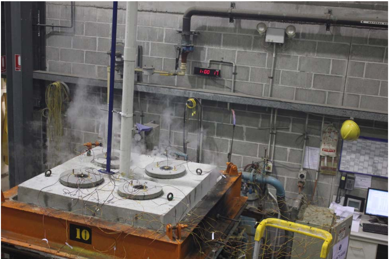
PHOTOGRAPH 3 – SPECIMENS AFTER 60 MINUTES OF TESTING
