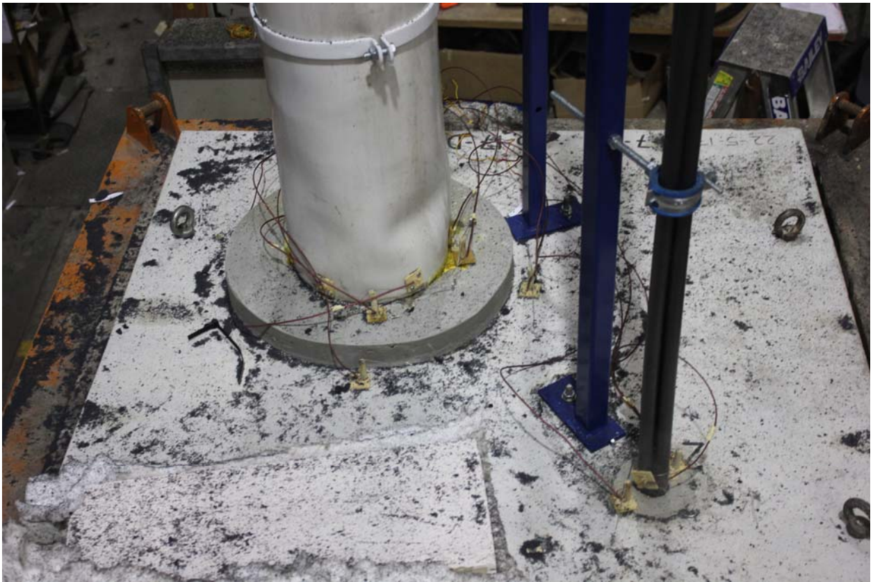
PHOTOGRAPH 5 – SPECIMENS AFTER 180 MINUTES OF TESTING
