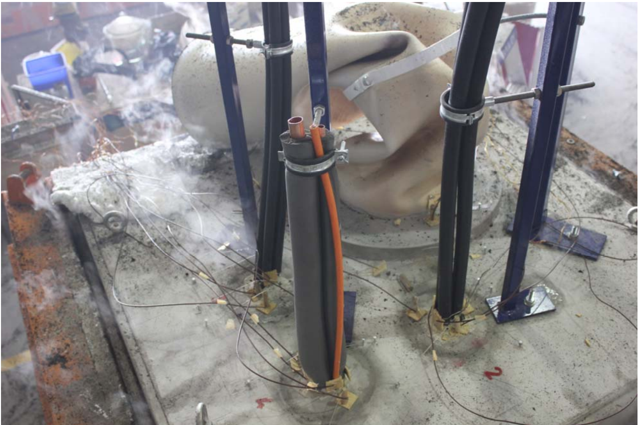
PHOTOGRAPH 5 – PENETRATIONS AFTER 60 MINUTES OF TESTING
