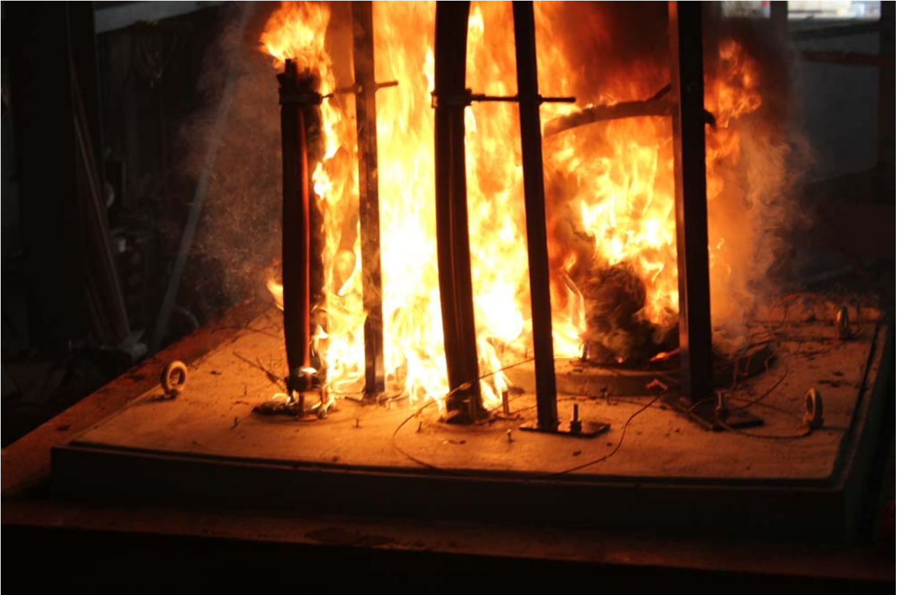
PHOTOGRAPH 8 – UNEXPOSED FACED OF PENETRATION AT CONCLUSION OF TESTING
