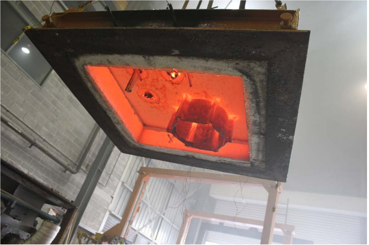
PHOTOGRAPH 9 – EXPOSED FACE OF PENETRATIONS AT CONCLUSION OF TESTING
