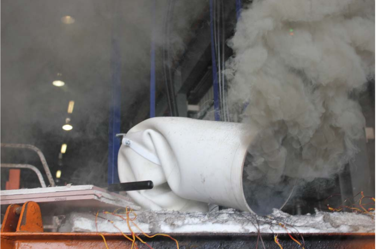
PHOTOGRAPH 3 – PENETRATION 1 AFTER 7 MINUTES OF TESTING
