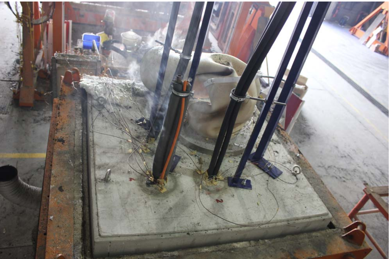
PHOTOGRAPH 6 – PENETRATIONS AFTER 120 MINUTES OF TESTING
