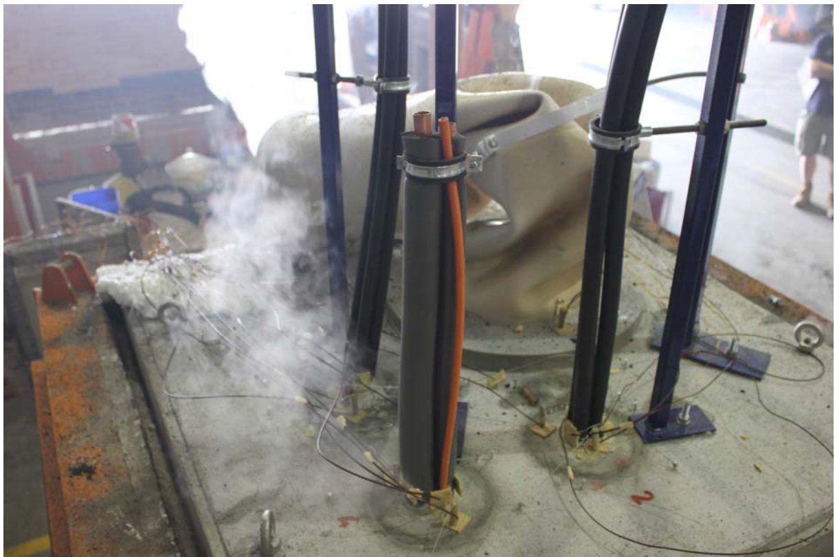
PHOTOGRAPH 4 – PENETRATIONS AFTER 30 MINUTES OF TESTING
