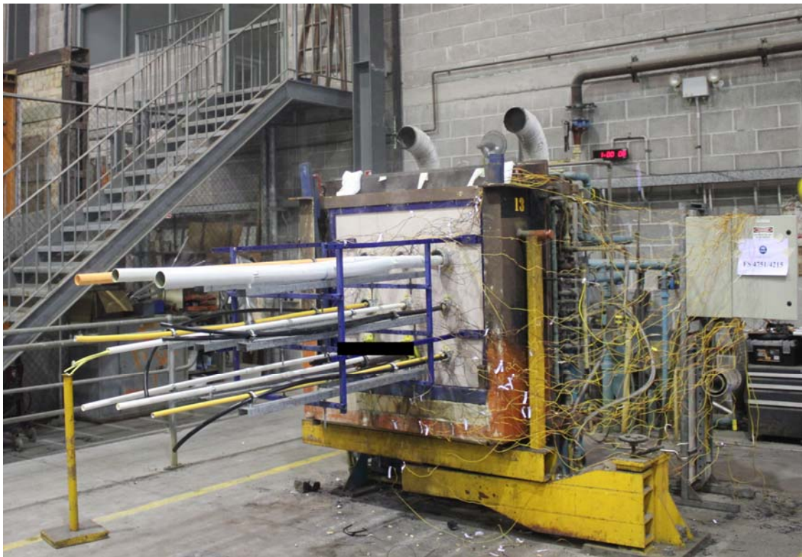
PHOTOGRAPH 4 – SPECIMENS AFTER 60 MINUTES OF TESTING
