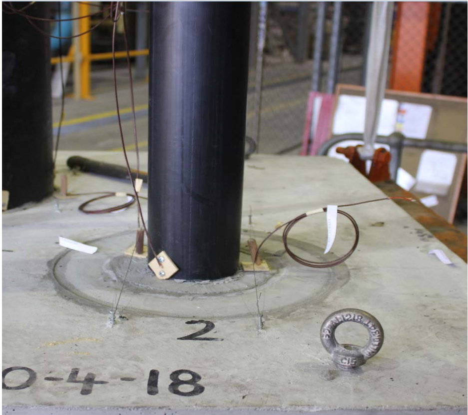
PHOTOGRAPH 2 – UNEXPOSED FACE OF SPECIMEN 2 PRIOR TO TESTING
