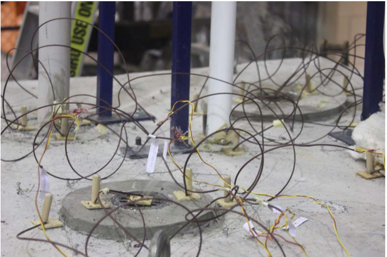
PHOTOGRAPH 11 – UNEXPOSED FACED OF SPECIMEN AT THE CONCLUSION OF TESTING
