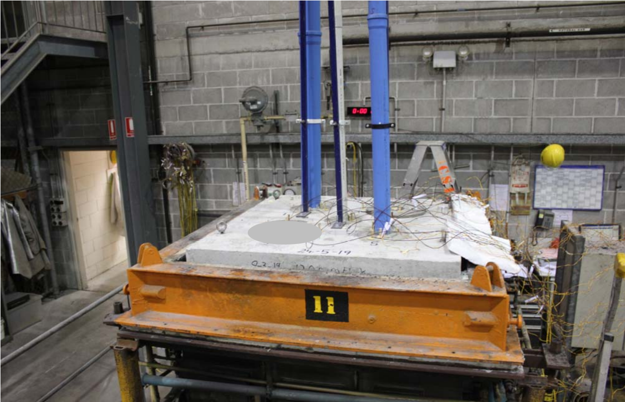
PHOTOGRAPH 2 – UNEXPOSED FACE OF SPECIMENS PRIOR TO TESTING
