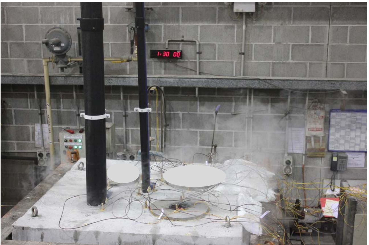
PHOTOGRAPH 6 – SPECIMENS AFTER 90 MINUTES OF TESTING
