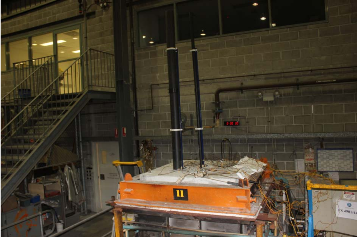
PHOTOGRAPH 2 – UNEXPOSED FACE OF SPECIMENS PRIOR TO TESTING
