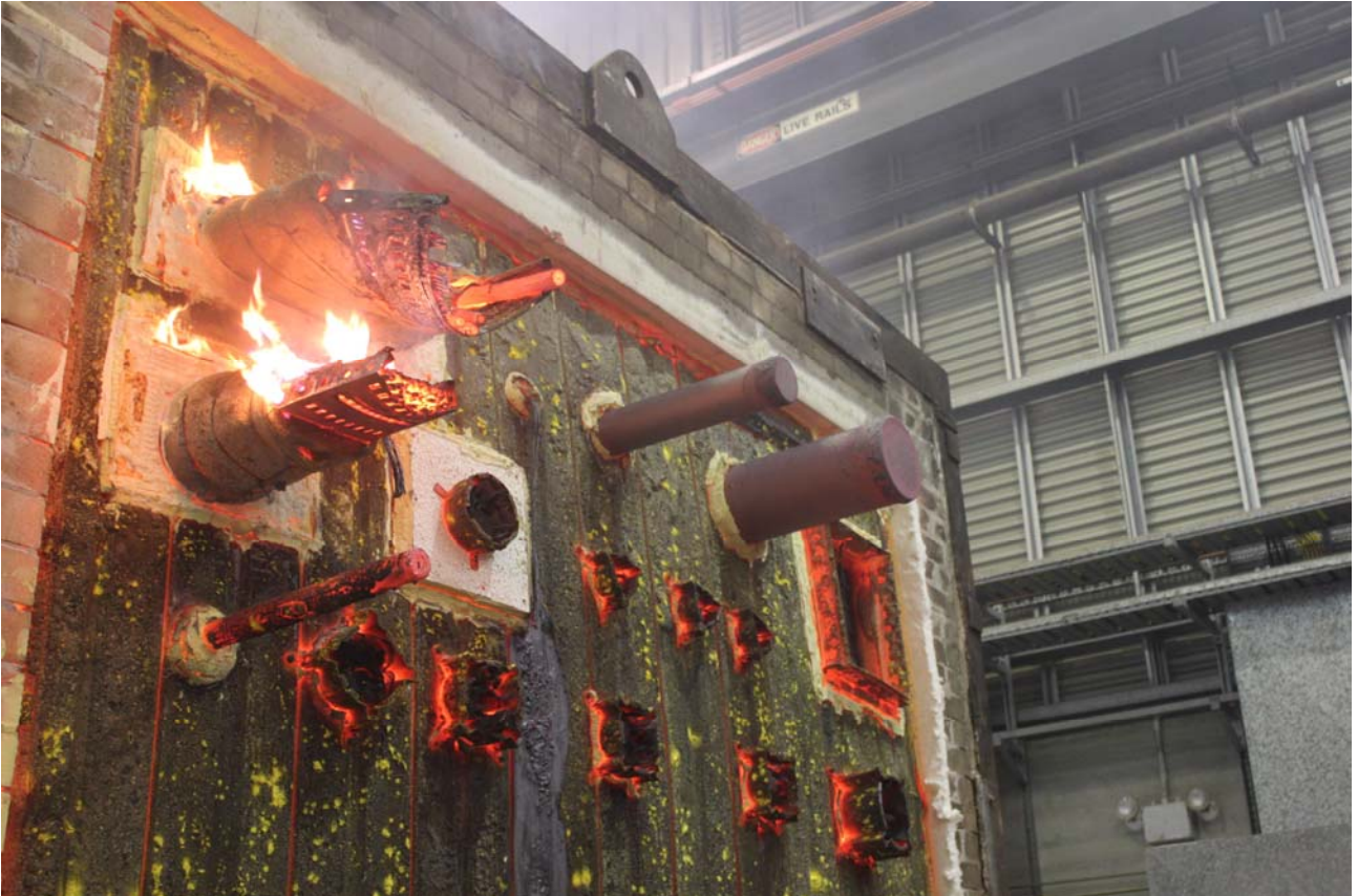
PHOTOGRAPH 14 – EXPOSED FACE OF THE SPECIMEN AFTER THE CONCLUSION OF TESTING
